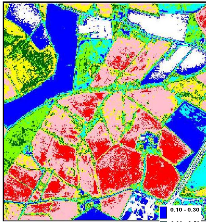
(a) IKONOS 4m true colour orthoimagery. (b) NDVI calculated from IKONOS 4m multispectral imagery.
