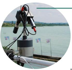
**So-Rad** (Solar-tracking radiometry platform) by **PML** providing water-leaving Reflectance (3 channels) integrating existing sensors, providing azimuth angle control. €2.5k to build (excl. sensors). Fully open-source.
